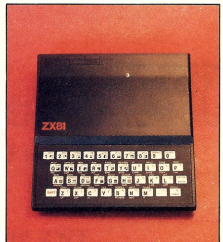
The ZX81 uses a standard home television for display and a tape cassette recorder for program storage. A 16K RAM attaches to the back of the computer.
